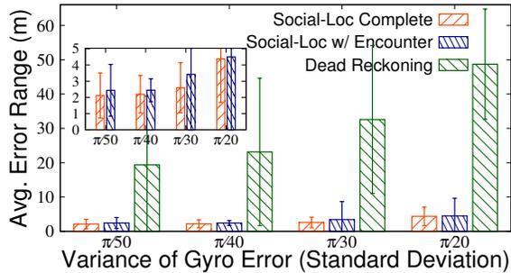
Figure 20: Variance of Gyroscope Error vs. Localization Error
