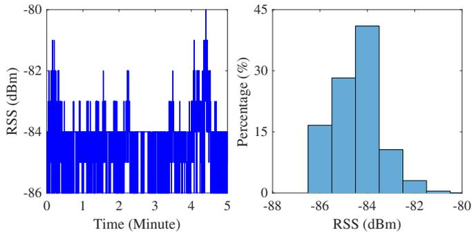
Fig. 2. RSS value of a UAV at a fixed location
