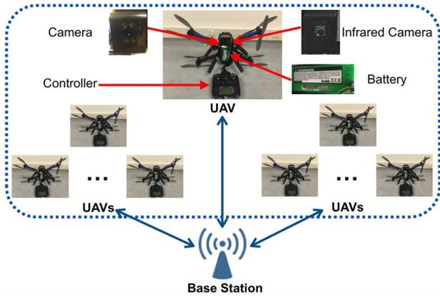
Fig. 1. A UAV network structure. Each UAV has one regular camera and one infrared camera.
