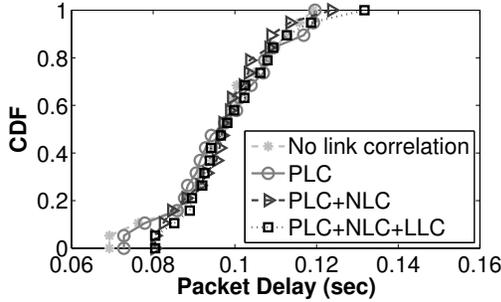
Fig. 12. Emulation results showing end-to-end packet delay for utilizing different link correlations
