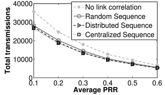
Fig. 17. Simulation results showing the effect of average PRR at macro-level
