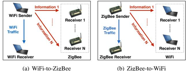
Fig. 1: Example of bi-directional EMF communication (i.e., WiFi to ZigBee and ZigBee to WiFi). Figure 1(a) shows that the WiFi sender can embed  $N$  pieces of information into its regular WiFi traffic and concurrently send out these information to  $N$  ZigBee receivers when the WiFi sender is communicating with the WiFi receiver. Similarly, Figure 1(b) shows the reverse direction.
