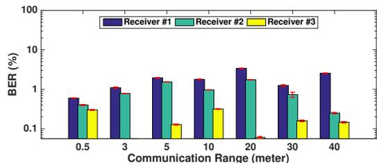
(b) BER (the Y-axis is in log scale)
