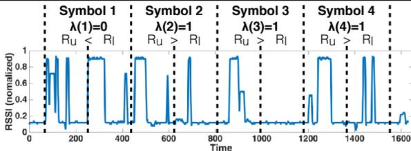
Fig. 9: An example of demodulation with empirical data lower half (shown in Figure 8(b)). Similarly, if the original packet-order yields  $\lambda = 0$ , but the sender wants to transmit “1”, the sender also can flip the packet(s) from the lower half to the upper half.
