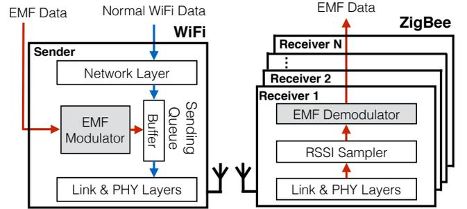
Fig. 4: Overview of WiFi to ZigBee EMF system architecture. By exchanging the terms “WiFi” and “ZigBee” in the above figure, we can also get the ZigBee to WiFi EMF system architecture.
