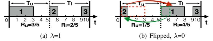
Fig. 8: An example of the flipping operation
