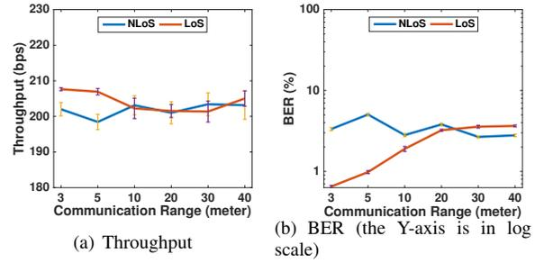
Fig. 14: Throughput and BER of one-to-one EMF: The performance in NLoS scenario is slightly lower than in LoS in most circumstances, but they are very close to each other when distance increases.
