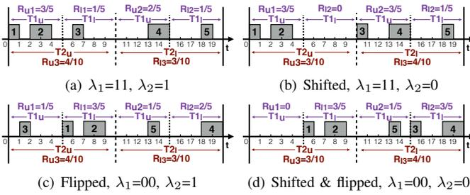
Fig. 11: An example of one-to-two modulation: two messages  $S1$  and  $S2$  are transmitted by using windows sizes 5 and 10, respectively. With different shifting and/or flipping operations for packets #1 to #5, arbitrary  $\lambda_1$  and  $\lambda_2$  can be transmitted. For example, in Figure 11(a), the original  $\lambda_2 = 1$ . In order to transmit  $\lambda_2 = 0$ , we need to shift packet #3 (shown in Figure 11(b)). More detailed combinations are shown in Table III.
