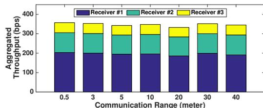
Fig. 18: Aggregated throughput of three ZigBee receivers: the highest aggregated is 356 bps at 0.5m communication range and the throughput is 344 bps at 40m.
