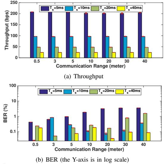
Fig. 15: Impact of window size  $T_s$ : The throughput is half when the window size  $T_s$  doubled (because the modulation mechanism we used) and it is very stable across all the communication range (from 0.5m to 40m) which shows our EMF modulation scheme is robust.
