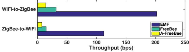
Fig. 13: Comparison between EMF and state-of-the-art cross technology communication FreeBee [1].
