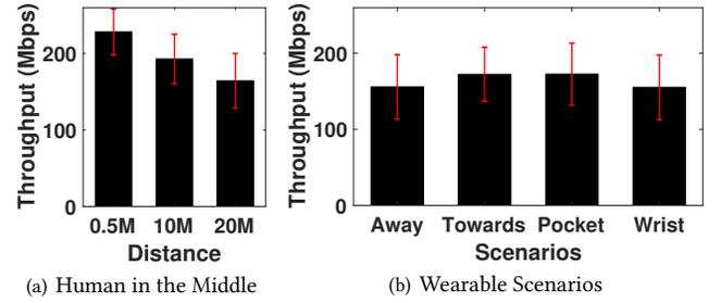
Figure 24: Gateway-to-WiFi Throughput in Mobile Scenarios: In human in the middle scenario, the Gateway-to-WiFi link's throughput can be up to 245.07 Mbps. In different wearable scenarios, our approach maintains similar throughput. This demonstrates that our design can support different types wearable applications.
