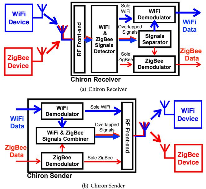
Figure 4: System Architecture
