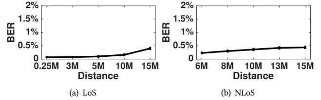
Figure 20: Bit Error Rate of Gateway-to-ZigBee Link: The BER remains low (less than 0.5%) even in NLoS scenario.
