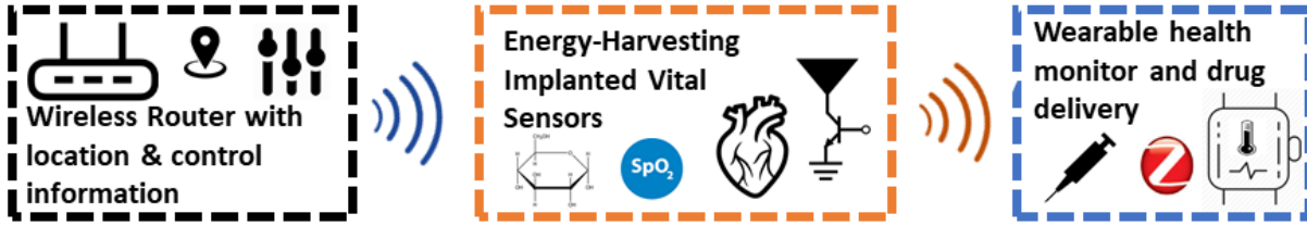
Figure 2: A health-monitoring application where WiFi router provides localization data and control messages relayed by Passive-ZigBee’s tag. This tag also sends glucose, oxygen saturation, and ECG data. The listener is a long-battery-life wearable ZigBee health monitoring and medicine delivery device.
