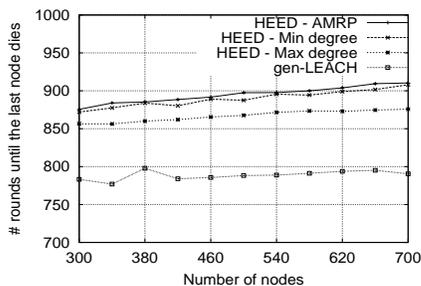
Fig. 9. Network lifetime using HEED and gen-LEACH (last node death)
