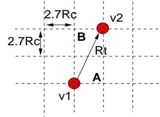
Fig. 4. Minimum transmission range for inter-cluster communication
