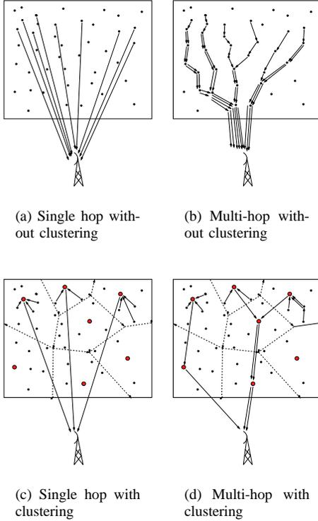
Fig. 1. Forwarding with and without clustering and aggregation
