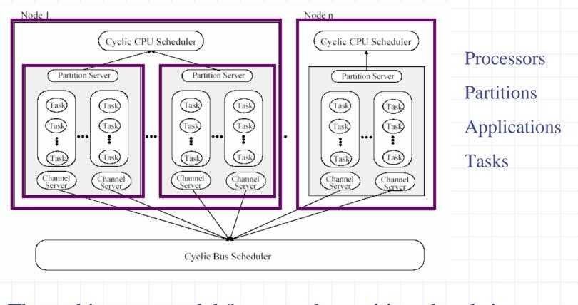
The architecture model for strongly partitioned real-time systems (SP-RTS)
