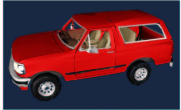
Plate 4: 26 pixels of screen-space error 9,000 triangles
