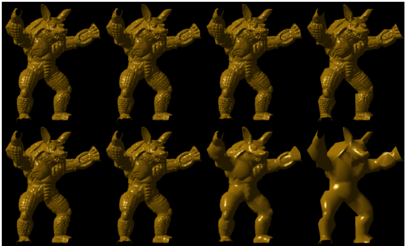
249,924 triangles 62,480 triangles 7,809 triangles 975 triangles 0.05 mm max image deviation 0.25 mm max image deviation 1.3 mm max image deviation 6.6 mm max image deviation
