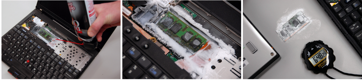
Figure 6: Before powering off the computer, we spray an upside-down canister of multipurpose duster directly onto the memory chips, cooling them to -50^{\circ}\text{C} . At this temperature, the data will persist for several minutes after power loss with minimal error, even if we remove the DIMM from the computer.
