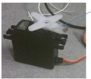
This is the light sensor, simply taped on, with wire wires going to the Butterfly
