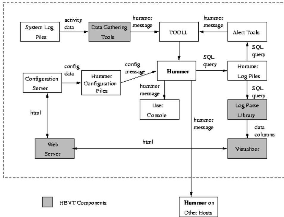
Figure 2: Hummingbird component interaction. Not shown: audit management and feature selection tools.
