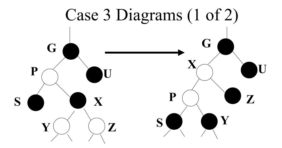
Step 1 – recolor X, Y and Z. Rotate X around P.
