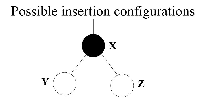
If new node is inserted as child of Y or Z, it's uncle will be red and we will have to go back up the tree. This is the only case we need to avoid.
