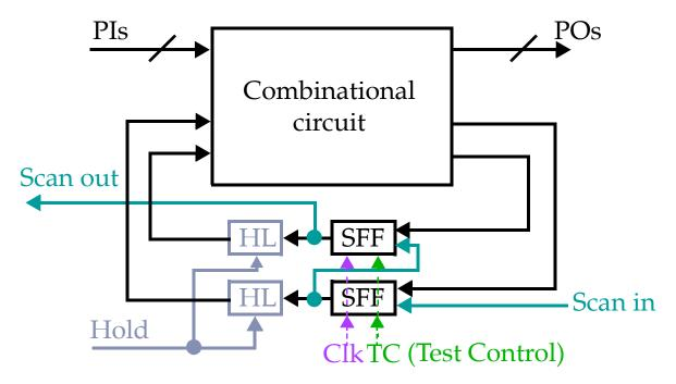
Each vector consists of two parts, bits for the PIs and bits for the state variables (SFFs).
