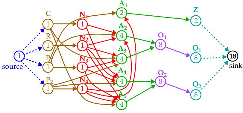
Vertices represent the PIs, POs and gates, edges represent signal flow.
