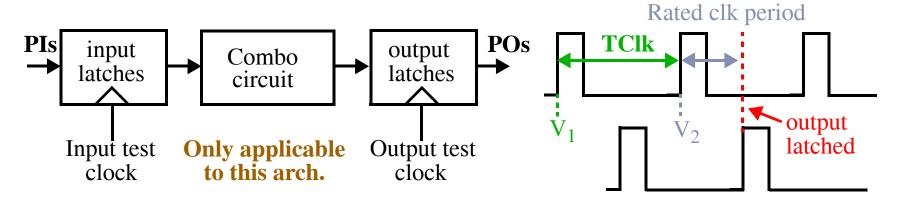
Note that  $V_1$  is applied at a slower rate and the circuit is allowed to stabilize.
