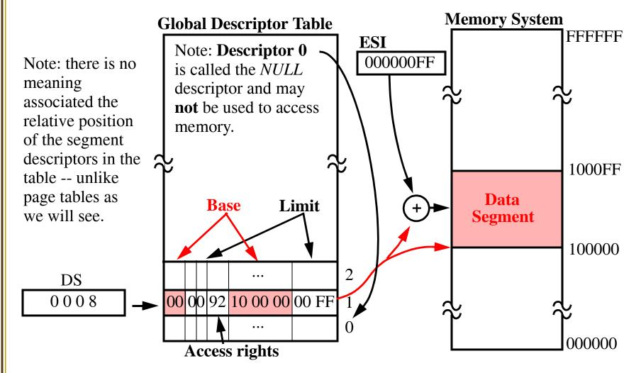
So instead of left shifting by 4 bits in Real Mode to form the segment address, we right shift by 3 bits and use the value as a table index.
