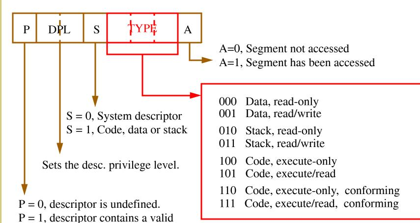
The Access Rights (AR) byte controls access to a protected mode segment and how the segment functions in the system.
