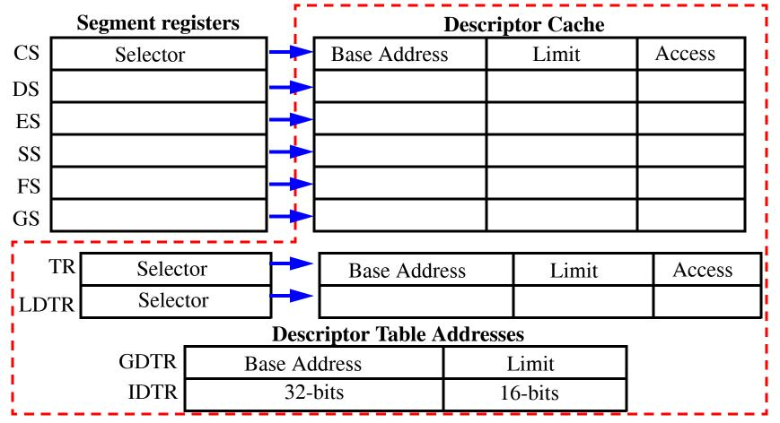
The addresses of the GDT and IDT and their limits (up to 64K bytes) are loaded in special registers, **GDTR** and **IDTR**, before switching to Protected Mode is possible.
