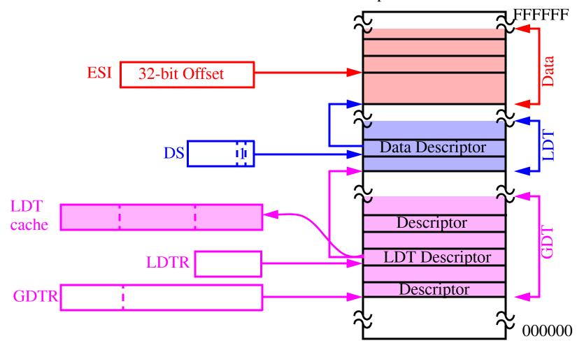
The LDTR selector can be loaded with a new value when another task is run.
