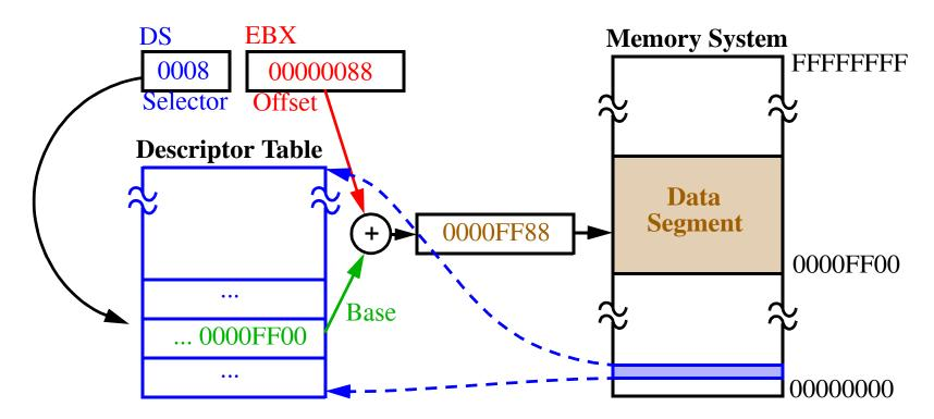
Segments are *interpreted* differently in Protected Mode vs. Real Mode:
