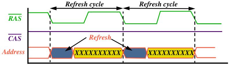
Simplest and most widely used method for refreshing, carry out a dummy read cycle
