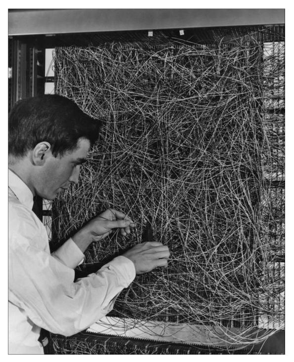
A man adjusting the random wiring network between the light sensors and association unit of scientist Frank Rosenblatt's Perceptron, or MARK 1 computer, at the Cornell Aeronautical Laboratory, Buffalo, New York, circa 1960. The machine is designed to use a type of artificial neural network, known as a perceptron. (Photo by Frederic Lewis/Archive Photos/Getty Images)
