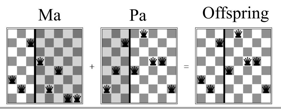
**Figure 4.7** The 8-queens states corresponding to the first two parents in Figure 4.6(c) and the first offspring in Figure 4.6(d). The shaded columns are lost in the crossover step and the unshaded columns are retained.
