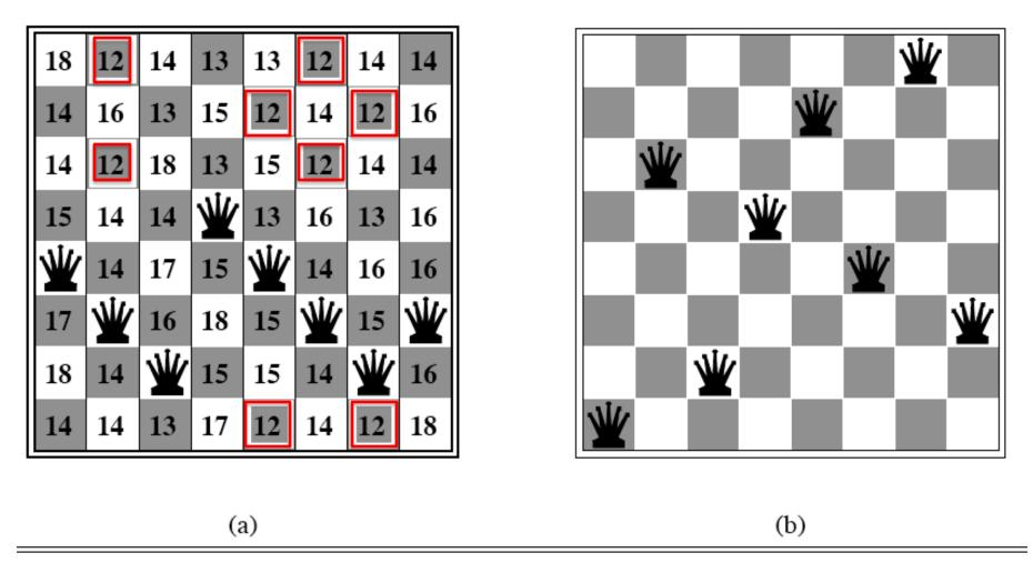
**Figure 4.3** (a) An 8-queens state with heuristic cost estimate h = 17, showing the value of h for each possible successor obtained by moving a queen within its column. The best moves are marked. (b) A local minimum in the 8-queens state space; the state has h = 1 but every successor has a higher cost.
