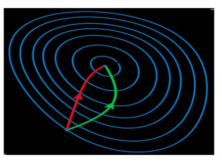
Contour lines of a function Gradient descent (green) Newton's method (red)
