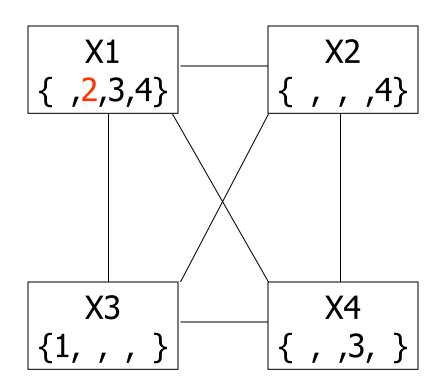
Arc constancy eliminates x3=3 because it's not consistent with X2's remaining values
