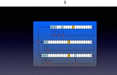
• Registers "step or stutter" according to a majority vote of the motion bits (orange).
