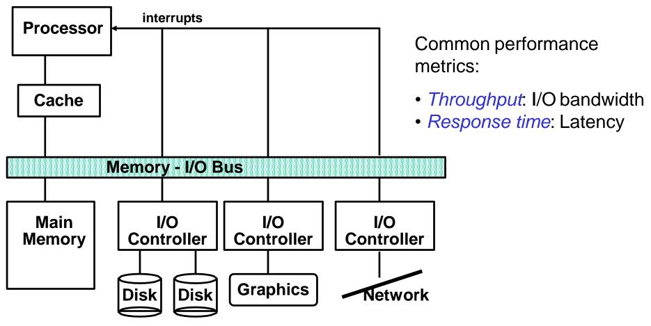
The connection between the I/O devices, processor, and memory are usually called (local or internal) <u>buses</u>
