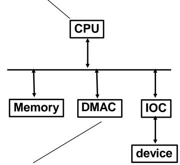
DMAC provides handshake signals for Peripheral Controller, and Memory Addresses and handshake signals for Memory.
