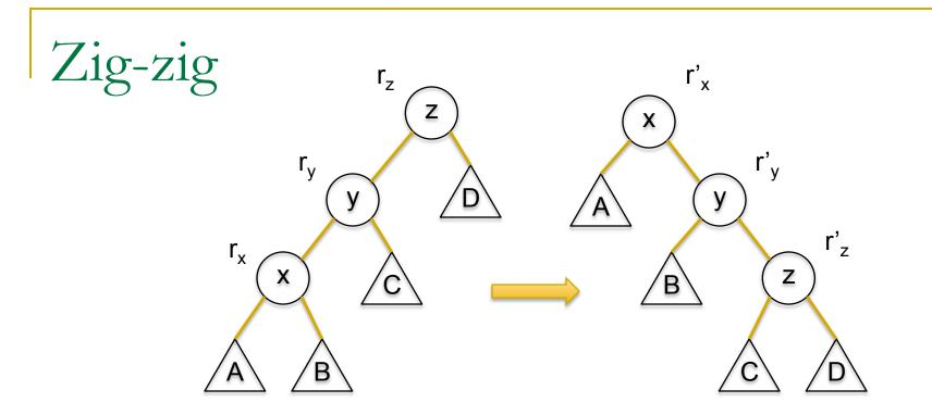
To maintain credit invariant at all nodes need to add  $\Delta = (r'_x - r_x) + (r'_y - r_y) + (r'_z - r_z)$ •Note that  $r'_x = r_z$  so ... • $\Delta = r'_y + r'_z - r_x - r_y$ •Note that  $r'_x \ge r'_y$  and  $r'_x \ge r'_z$  and  $r_x \le r_y$  so ... • $\Delta = r'_y + r'_z - r_x - r_y \le r'_x + r'_x - r_x - r_x = 2(r'_x - r_x)$
