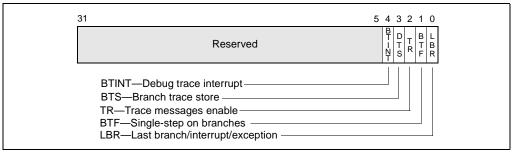
Figure 14-2. IA32\_DEBUGCTL MSR (Pentium 4 Processors)
