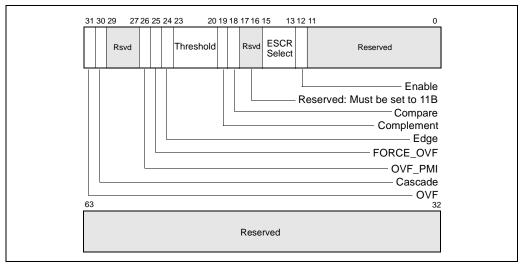
Figure 14-9. Counter Configuration Control Register (CCCR)
