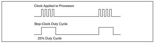
Figure 12-6. Processor Modulation Through Stop-Clock Mechanism
