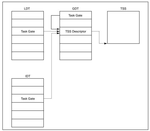
Figure 6-6. Task Gates Referencing the Same Task
