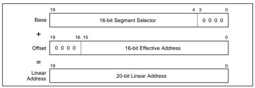
Figure 15-1. Real-Address Mode Address Translation
