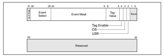
Figure 14-7. Event Selection Control Register (ESCR) (Pentium 4 Processors)
