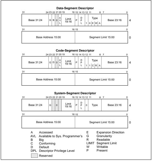
Figure 4-1. Descriptor Fields Used for Protection
