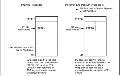
Figure 17-1. I/O Map Base Address Differences
