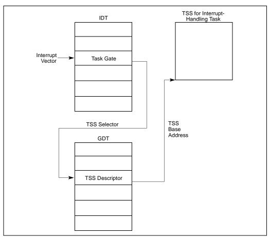
Figure 5-5. Interrupt Task Switch
