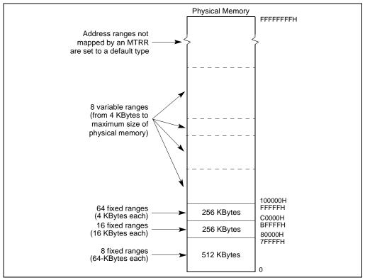
Figure 9-3. Mapping Physical Memory With MTRRs
