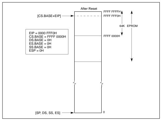
Figure 8-3. Processor State After Reset
