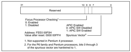
Figure 7-15. Spurious-Interrupt Vector Register (SVR)
