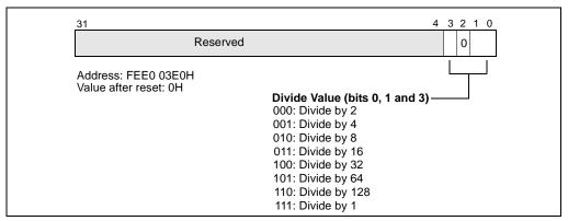
Figure 7-18. Divide Configuration Register
