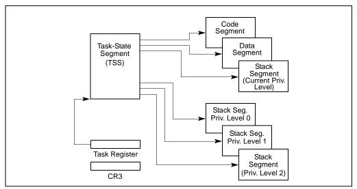
Figure 6-1. Structure of a Task
