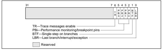
Figure 14-6. DebugCtIMSR Register (P6 Family Processors)
