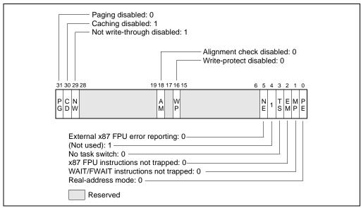
Figure 8-1. Contents of CR0 Register after Reset
