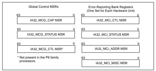
Figure 13-1. Machine-Check MSRs
