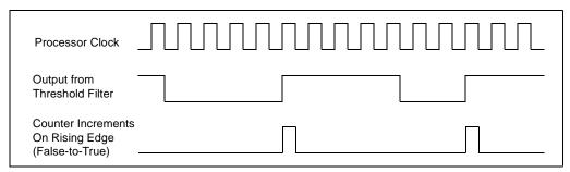
Figure 14-14. Effects of Edge Filtering
