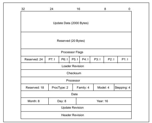
Figure 8-8. Format of the Microcode Update Data Block
