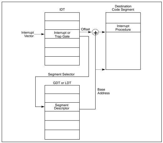
Figure 5-3. Interrupt Procedure Call
