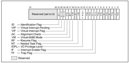
Figure 2-3. System Flags in the EFLAGS Register
