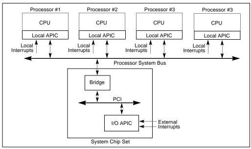
Figure 7-2. Local APICs and I/O APIC When Pentium 4 Processors Are Used in Multiple-Processor Systems
