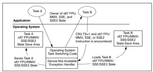
Figure 11-1. Example of Saving the x87 FPU, MMX, SSE, and SSE2 State During an Operating-System Controlled Task Switch
