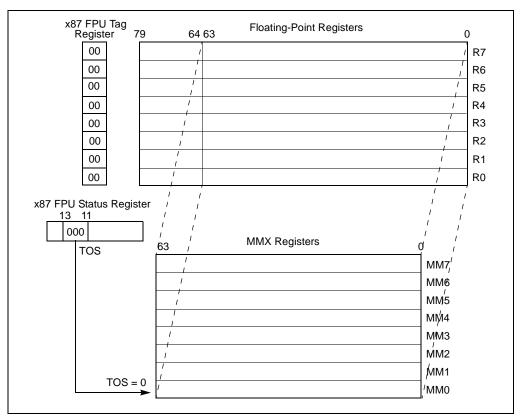
Figure 10-1. Mapping of MMX Registers to Floating-Point Registers
