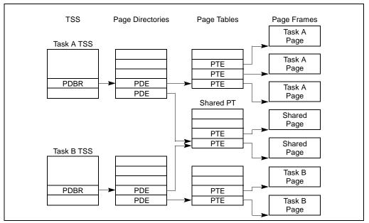
Figure 6-8. Overlapping Linear-to-Physical Mappings
