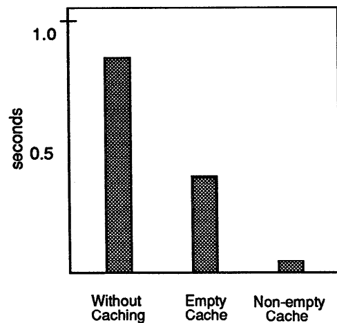
Figure 5: Cache performance is measured for three cases: (a) the without caching or base-line case where caching was disabled, (b) the empty cache case where caching was enabled but the cache was cleared before each repetition of the test set, and (c) the non-empty cache case where the cache contained the results for all queries in the test set.
