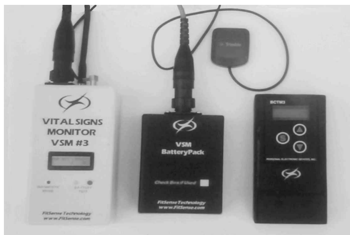
FIG. 2. The vital-signs monitoring (VSM) system of FitSense, Inc., demonstrating (right to left) the global positioning satellite (GPS) module, the central processing hub, and the radio frequency (RF) transmitter. (Courtesy of Dr. Tom Blackadar, Ph.D., FitSense Technologies, Inc., Wellesley, Massachusetts.)
