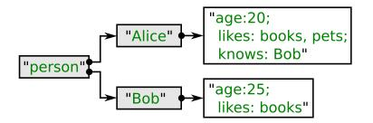
**Figure 1.3:** Example data represented in a wide column store. Here "person" is used as column key and each person's name as row key. Like in a Key-Value store, the stored value is not further interpreted by the system.
