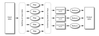
**Figure 1.6:** Model of the MapReduce framework. The split input data is handed to several processes running the MAP function. Return values of the map functions are combined to intermediate results. For each intermediate result, one REDUCE process is executed.
