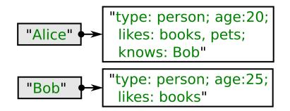
**Figure 1.2:** Example data represented in a Key-Value store. The stored value (here of type String) typically can not be interpreted by the storage system.
