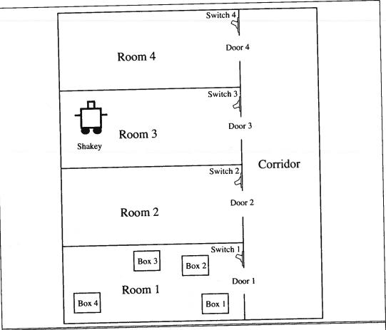
Figure 10.14 Shakey's world. Shakey can move between landmarks within a room, can pass through the door between rooms, can climb climbable objects and push pushable objects, and can flip light switches.
