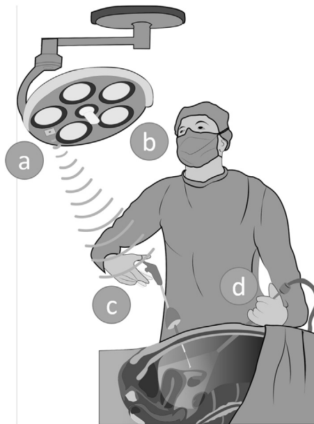
Fig. 5. No hands interaction: RadSense attached to medical light (a), viewing image (b), performing finger gesture while holding a tool (c) busy hand holding tool (d).
