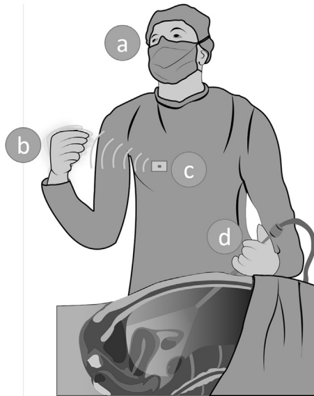
Fig. 4. One hand interaction: viewing the image (a), performing a gesture (b), RadSense worn on chest (c) busy hand holding tool (d).
