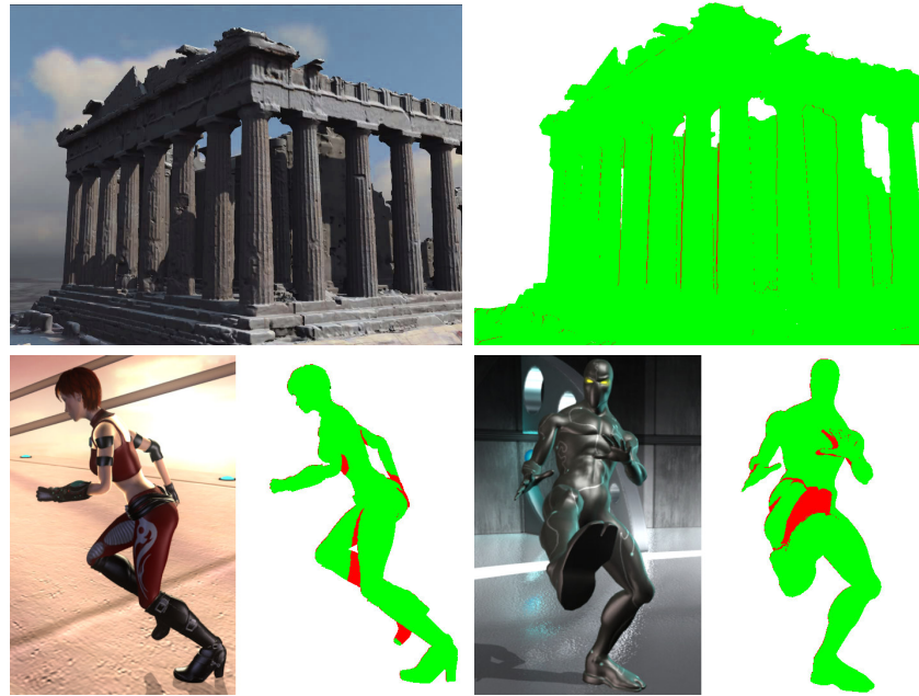
Figure 6.1: Real-time rendering applications exhibit a considerable amount of spatio-temporal coherence. This is true for camera motions (top) as well as for animated object (bottom). The snapshots of the Parthenon, Heroine, and Ninja sequences illustrate this fact. Newly visible surface points are rendered in red, whereas the vast majority (shown in green) were previously visible. We introduce a real-time method that exploits this coherence by caching and tracking visible surface information.
