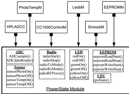
**Figure 4: Wiring of the PowerState module.** Each hardware component is wired to the PowerState module as shown in the figure. Whenever a power state change occurs the corresponding command in PowerState is invoked to generate a state transition message.
