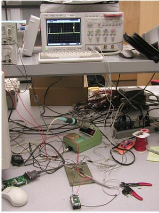
**Figure 1: Our hardware measurement configuration.** Our setup includes an oscilloscope, instrumentation amp, power supply, mote, PC, and programming board. The instrumented mote is at the bottom center of the picture.
