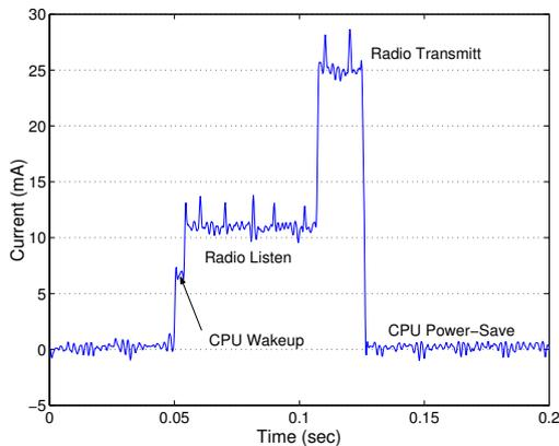
**Figure 2: Measured current consumption for transmitting a single radio message at maximum transmit power on the Mica2 node.**
