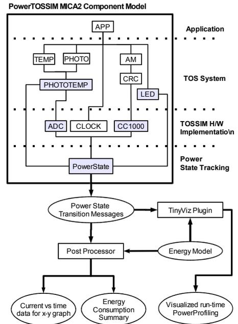
**Figure 3: PowerTOSSIM architecture.** *Simulated hardware components (radio, sensors, LEDs, etc.) make calls to the PowerState module, which emits power state transition messages for each component. These messages can be combined with a power model to generate detailed power consumption data or visualizations. (AM is the active messaging component that makes up the upper level of the radio stack)*
