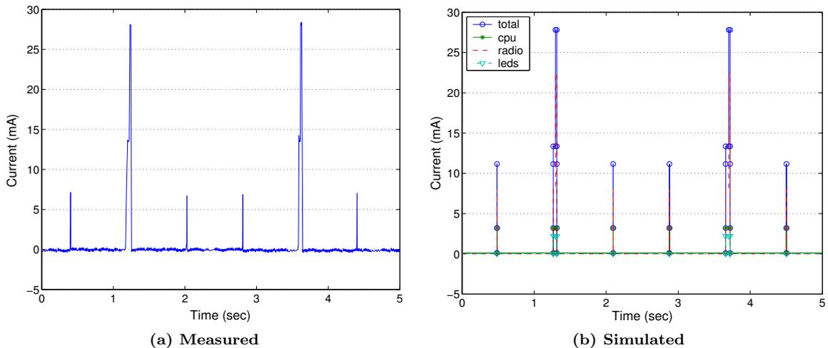
Figure 6: Measured and simulated current consumption for the *Beacon* application. The simulated version includes a breakdown according to radio, LEDs, and CPU current. A lower resolution digital multi-meter was used for the above measurement, which did not capture the very short duration peak power spikes during the wakeups.
