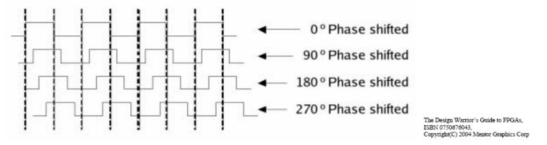
Common phase shifts are 120 and 240 degrees (for 3-phase clk schemes) and 90, 180 and 270 degrees for 4-phase schemes.
