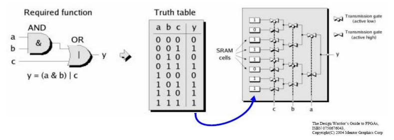
Input signals can be decoded using a hierarchy of transmission-gate MUXs.
