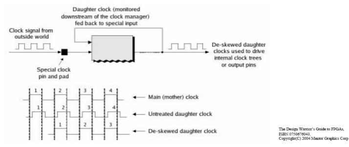
Skew in the daughter is removed by comparing it with the external clk and delaying it until the edges re-align.
