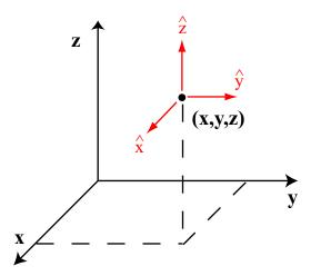
Figure 3.1: The rectangular coordinate system.
