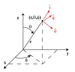
Figure 3.3: The spherical coordinate system.
