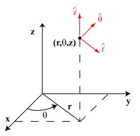
Figure 3.2: The cylindrical coordinate system.
