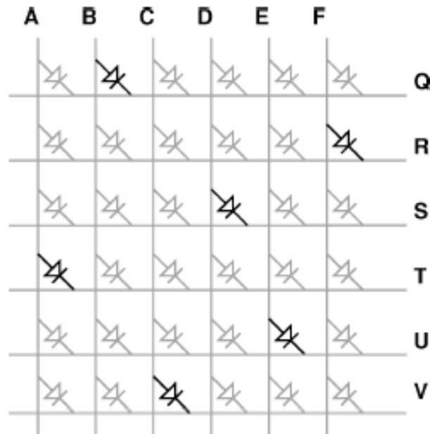
Fig. 7. Example crossbar routing configuration. Programmed on crosspoints are shown in black; off crosspoints are shown in grey. Here we show the crossbar programmed to connect A \rightarrow T , B \rightarrow Q , C \rightarrow V , D \rightarrow S , E \rightarrow U , and F \rightarrow R .
