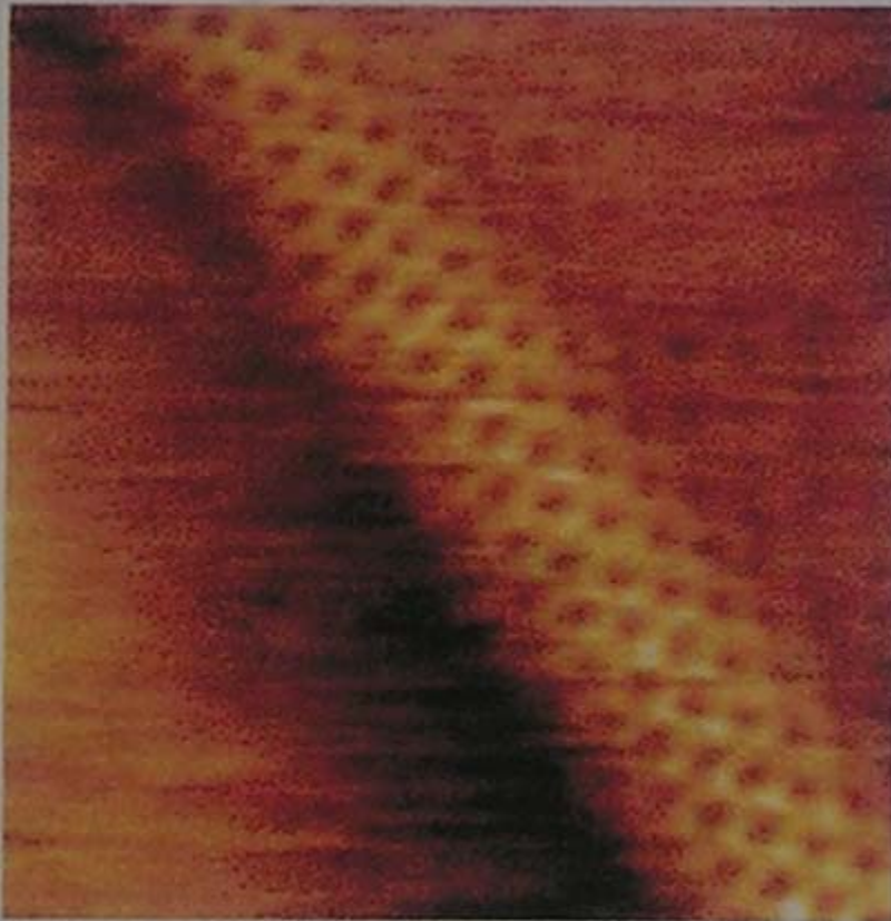
Figure 5: STM image at 77 K of a SWNT at the surface of a rope [6].
