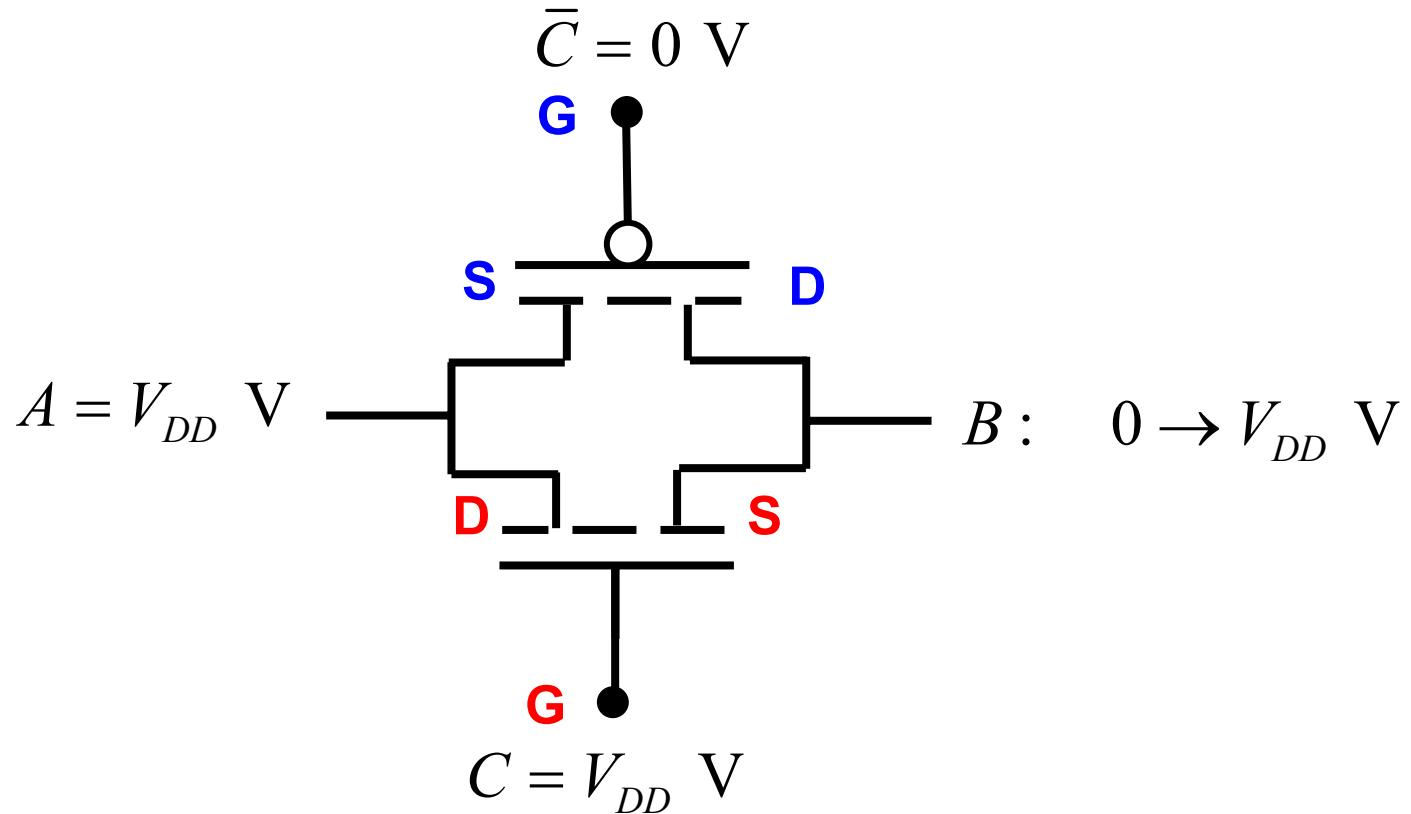
PMOS can charge the output all the way to  $V_{DD}$  V;
