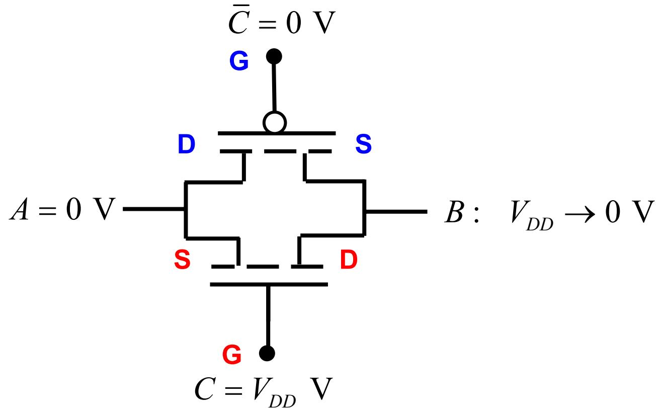
NMOS can discharge the output all the way to 0V;
