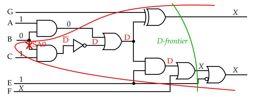
• Forward implication: Results when the inputs to a logic gate are labeled so that the output can be uniquely determined.
