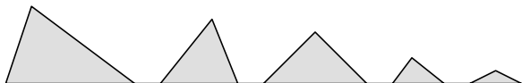
Figure 12: Step 2 rotates and translates triangles in the plane to place their longest edge along the x-axis, and Step 3 sorts these triangles by decreasing altitude.
