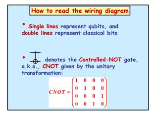
How to read the wiring diagram
