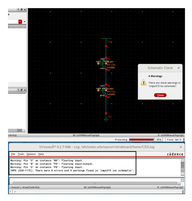
Figure 14: Schematic errors & warnings
