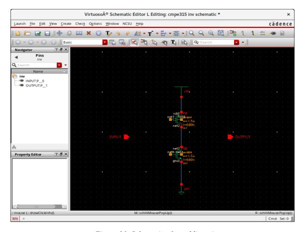
Figure 16: Schematic after adding pins
