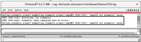
Figure 18: CIW showing no errors/warnings after Check & Save
