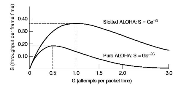
The maximum throughput occurs at G = 0.5 and the value of throughput is 0.18 (approximately), i.e., 82% of frames end up in collisions and are therefore lost.
