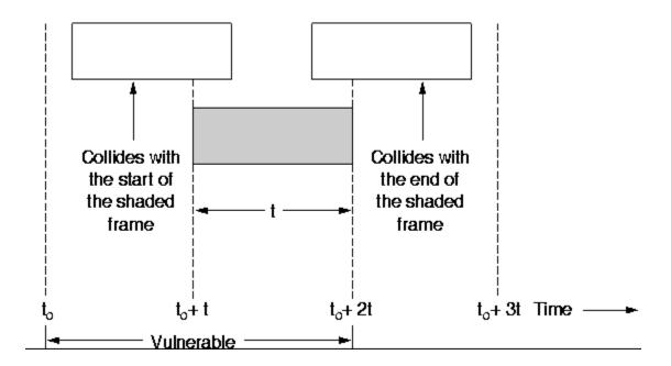
If the shaded frame has been sent (above), under what conditions will the shaded frame arrive intact? Let t be the time to send a frame - if another user has sent a frame between to and to + t, the end of the frame will collide with the shaded one. Similarly on the right side of the shaded frame - any frame that began between to + t and to + 2t will have an overlap with the end of the shaded frame. Therefore the **vulnerable period** is 2t - or two frame times.
