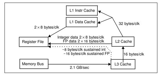
The register file can handle up to 2 integer register fills or 2 floating point register fills per clock from the caches.
