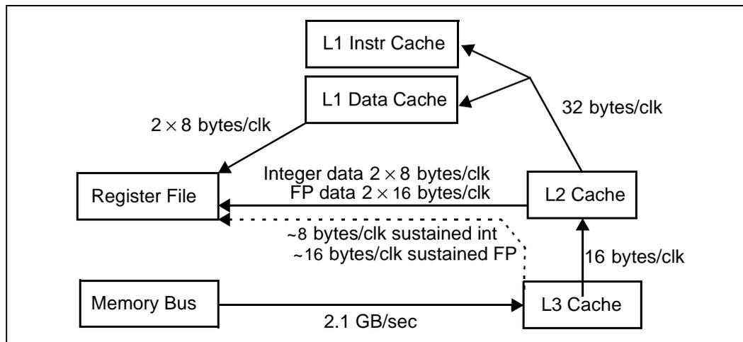
The register file can handle up to 2 integer register fills or 2 floating point register fills per clock from the caches.
