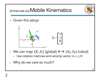
(A final note on) **Mobile Kinematics** (Final note on) **Mobile Kinematics** • Goal: take robot from A<sub>I</sub> to B<sub>I</sub> • We know where we want it in the global setting • What do we actually control? (In what frame of reference?) •  $\int_{y_1}^{y_2} \int_{y_2}^{y_3} \xi_A = \begin{pmatrix} x \\ y \\ \theta \end{pmatrix}$ • Point: Convert from A<sub>I</sub> to B<sub>I</sub> by changing  $\xi_R$
