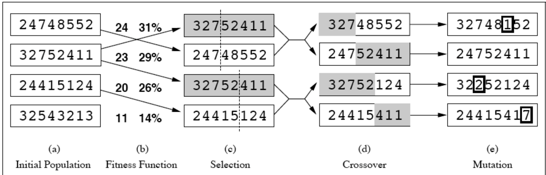
Figure 4.6 The genetic algorithm, illustrated for digit strings representing 8-queens states. The initial population in (a) is ranked by the fitness function in (b), resulting in pairs for mating in (c). They produce offspring in (d), which are subject to mutation in (e).
