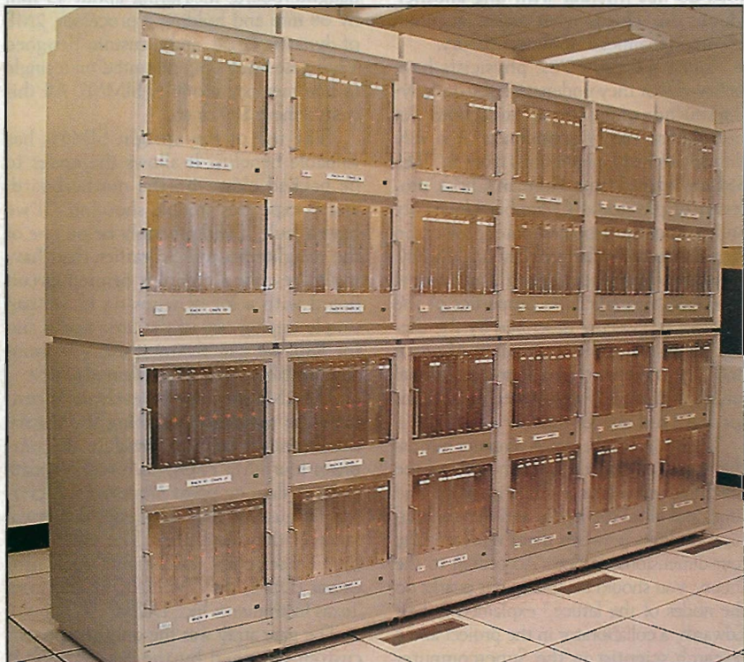
The 12 288-node supercomputer [above], capable of performing 0.6 trillion floating point operations per second, was built for only US $1.85 million. Physicists from Columbia University and other institutions developed the machine to simulate interactions among elementary particles called quarks and gluons. They received the 1998 Gordon Bell prize for price/performance.
