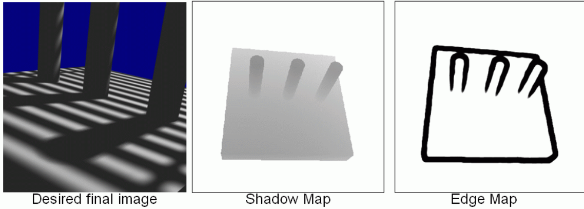
Figure 5 – The desired final image with soft shadows, the shadow map, and the edge map used for computation masking
