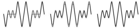
Figure 2: Comparison of computed (light) and sampled (dark) noise for different texture sizes: 2 samples/unit = texture size 2 \times \text{period} ; 3 samples/unit = texture size 3 \times \text{period} ; or 4 samples/unit = texture size 4 \times \text{period} .
