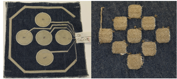
Fig. 8. As future work, we are exploring different capacitor plate shapes and placement. The left figure shows circular plates with a boundary plate that can be used to determine whether the user's is performing a gesture. The right figure demonstrates a future prototype where we plan to design the capacitive array using embroidered patches built using conductive threads.
