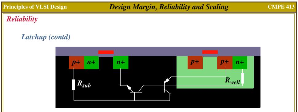
The cross-coupled transistors form a bistable silicon-controlled rectifier (SCR)
